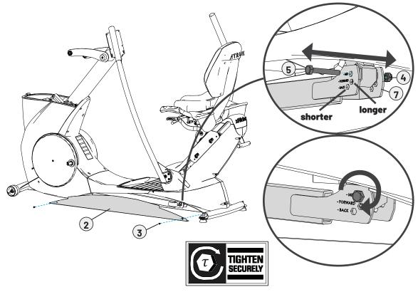
when using a torque wrench  $\mathcal{T}$  = 40 N-M (30 FT-LB)
