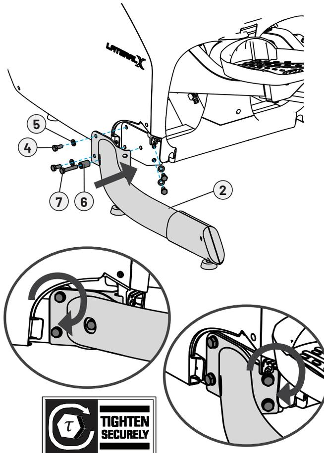
when using a torque wrench
