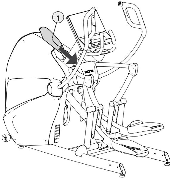
B. Attach one left and one right frame end cover around each frame end and secure in place using six M5 screws (3 per side).
